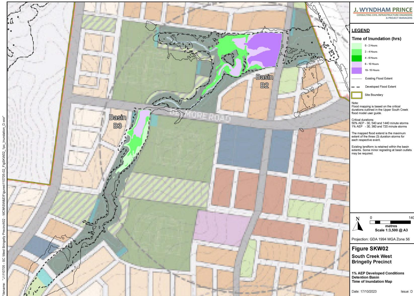
Figure 5-2: Detention basin time of inundation map for 1% AEP developed conditions (J. Wyndham Prince, 2023)
