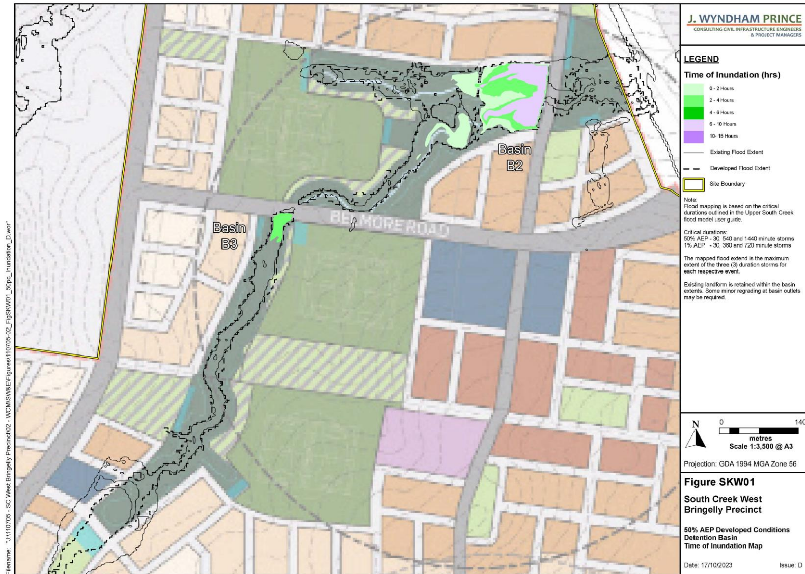
Figure 5-1: Detention basin time of inundation map for 50% AEP developed conditions (J. Wyndham Prince, 2023)
